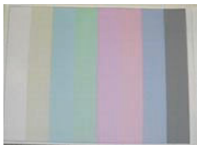
Conventional IR camera without IR-cut filter distorts the image color
